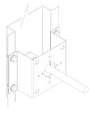
Orientation of Stand Off Bracket for a directly driven damper
